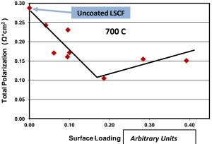
The Total Polarization resistance results for all samples tested during Phase I; at 600 C, 700 C, and 800 C. In all tests, the surface functionalized powders outperform the uncoated LSFC powder, as indicated by lower polarization resistance. The figures indicate there is an optimum surface loading.
