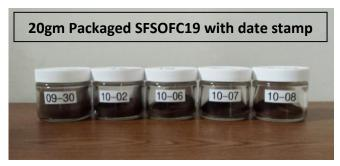
materials for functionalization coatings. SFSOFC19 uses 0.7 µm average particle size, La<sub>0.6</sub>Sr<sub>0.4</sub>Co<sub>0.2</sub>Fe<sub>0.8</sub>O<sub>3-δ</sub> (LSCF) for the base material powder. The first image shows uncoated material (left) and a typical powder after surface functionalization by the SMI process on the right. The second image shows packaged SFSOFC19 sample powder.
