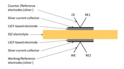
The cathode coated discs were sintered at 1000 C for 3 hours. Silver paste was applied, and used as the current collector. Electrochemical Impedance Spectroscopy (ESI) was done to characterize the electrochemical performance of the symmetrical cells under open circuit potential. Four probe tests were performed at 800 C, 700 C and 600 C in air.
