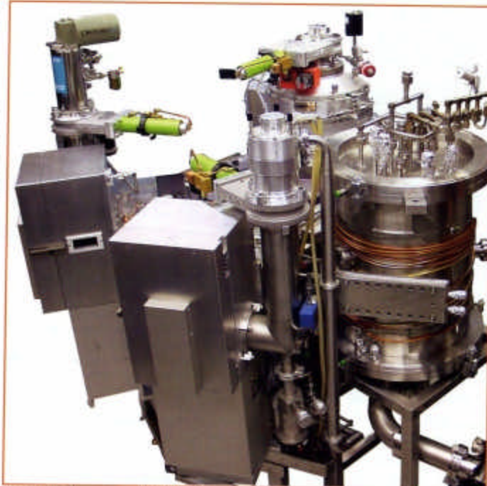
Figure 10. The rotating disk MOCVD reactor mounted in a cluster tool arrangement, along with an etch module and cassette-to-cassette load-locks.
