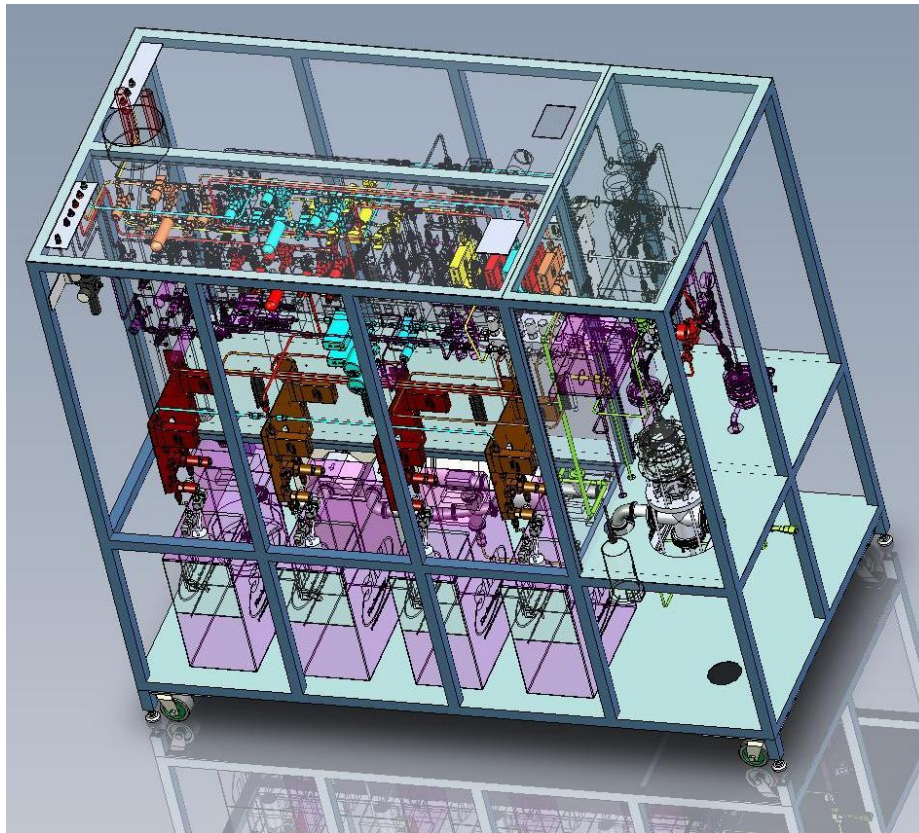
Figure 1 - Structured Materials Industry's pulsed MOCVD system. Four precursor handling systems are in the front reactor stays on the stage in the right front end the system.
