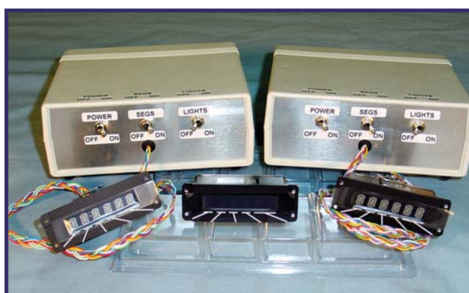
Figure 3: Prototype display devices fabricated with ZnO transparent conducting oxide coatings on the glass faceplates.
