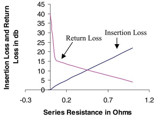
**Figure 6.** Variation of maximum insertion loss and return loss with series resistance. (See Color Plate XIII)
