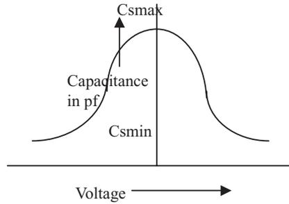
**Figure 3.** Capacitance versus voltage characteristics of a typical BST Capacitor.
