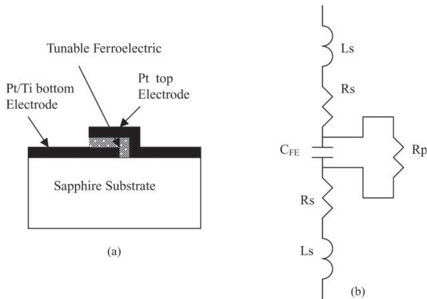
**Figure 4.** (a) Structure of tunable capacitor (b) Electrical equivalent circuit incorporating series resistance ( $R_s$ ), and inductance ( $L_s$ ) of top and bottom electrodes, as well as  $R_p$ , which is the parallel conductance of the tunable capacitor  $C_{FE}$ .
