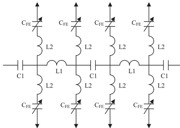
**Figure 2.** Schematic of lumped element band pass filter without incorporating parasitics.
