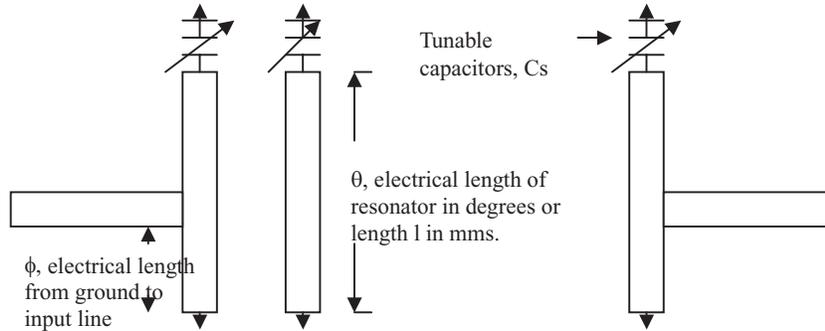
**Figure 1.** Schematics of distributed type band pass filter.
