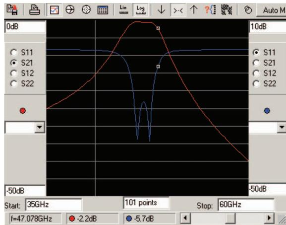
**Figure 8.** Response of the filter for 60% tunability of the ferroelectric capacitor. (See Color Plate XV)
