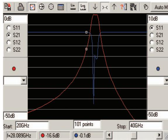
**Figure 5.** Simulated response of Ka band filter, showing the insertion loss and return loss. (See Color Plate XII)
