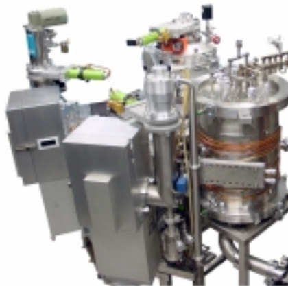
Fig. 13. Photograph of SMI cluster tool with one CVD tool and one etch tool.
